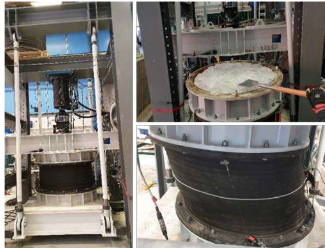
Large-scale simple shear test
