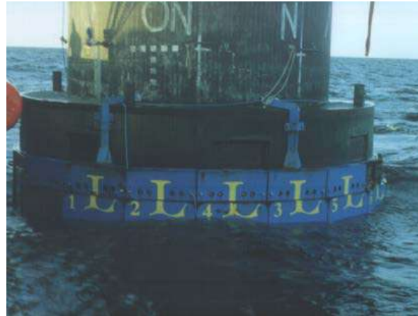
Ice-structure interaction load events on Norströmsgrund lighthouse
